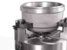
● Brake drum (truck) held in fixture
